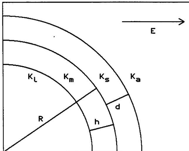
FIGURE 1 Schematic representation of the model used to represent a cell suspended in an electrolyte.
